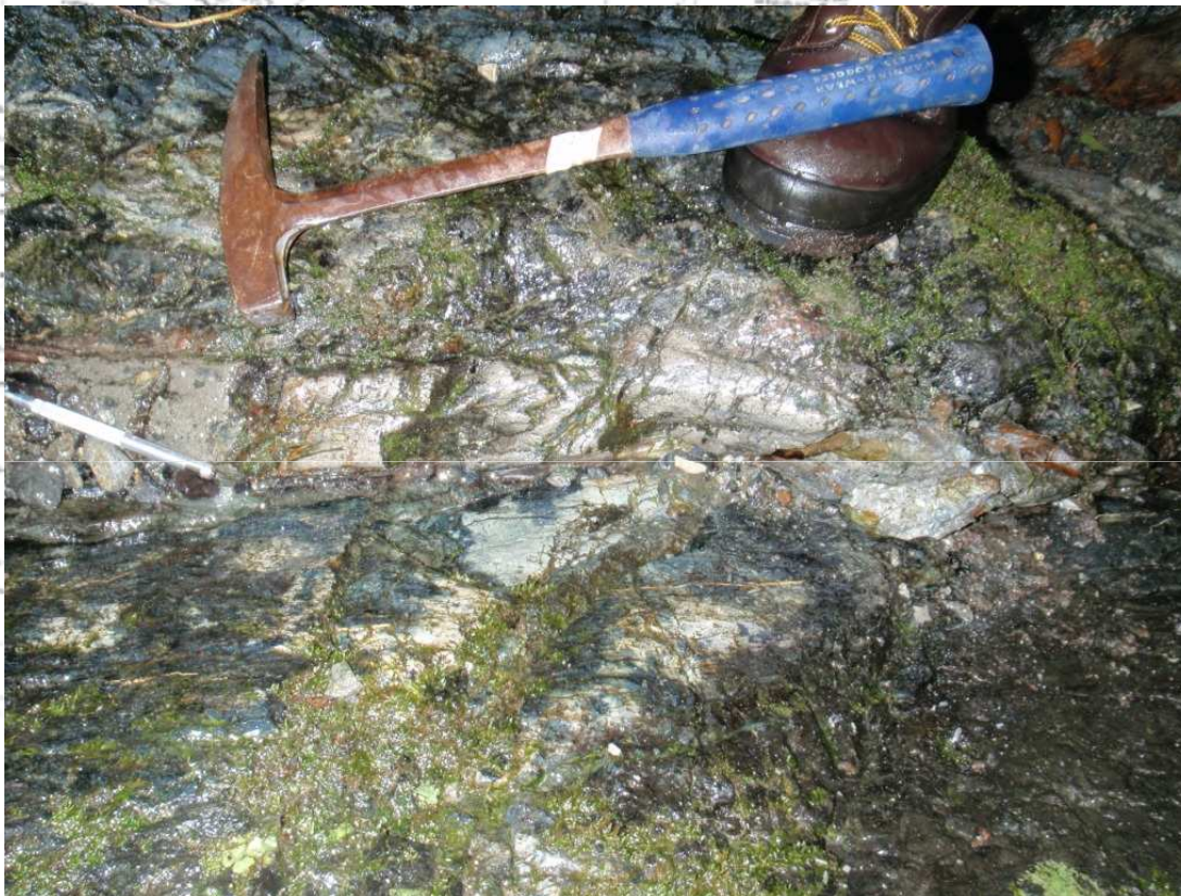
Iyewe Creek massive sulphide vein outcrop, 10-15cm thick
